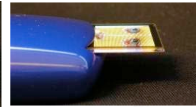
1.1" OLED displays of ca. 0.7 mm thin
