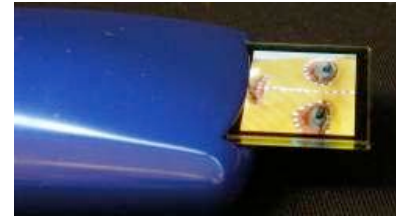
1.1" OLED displays of ca. 0.7 mm thin
